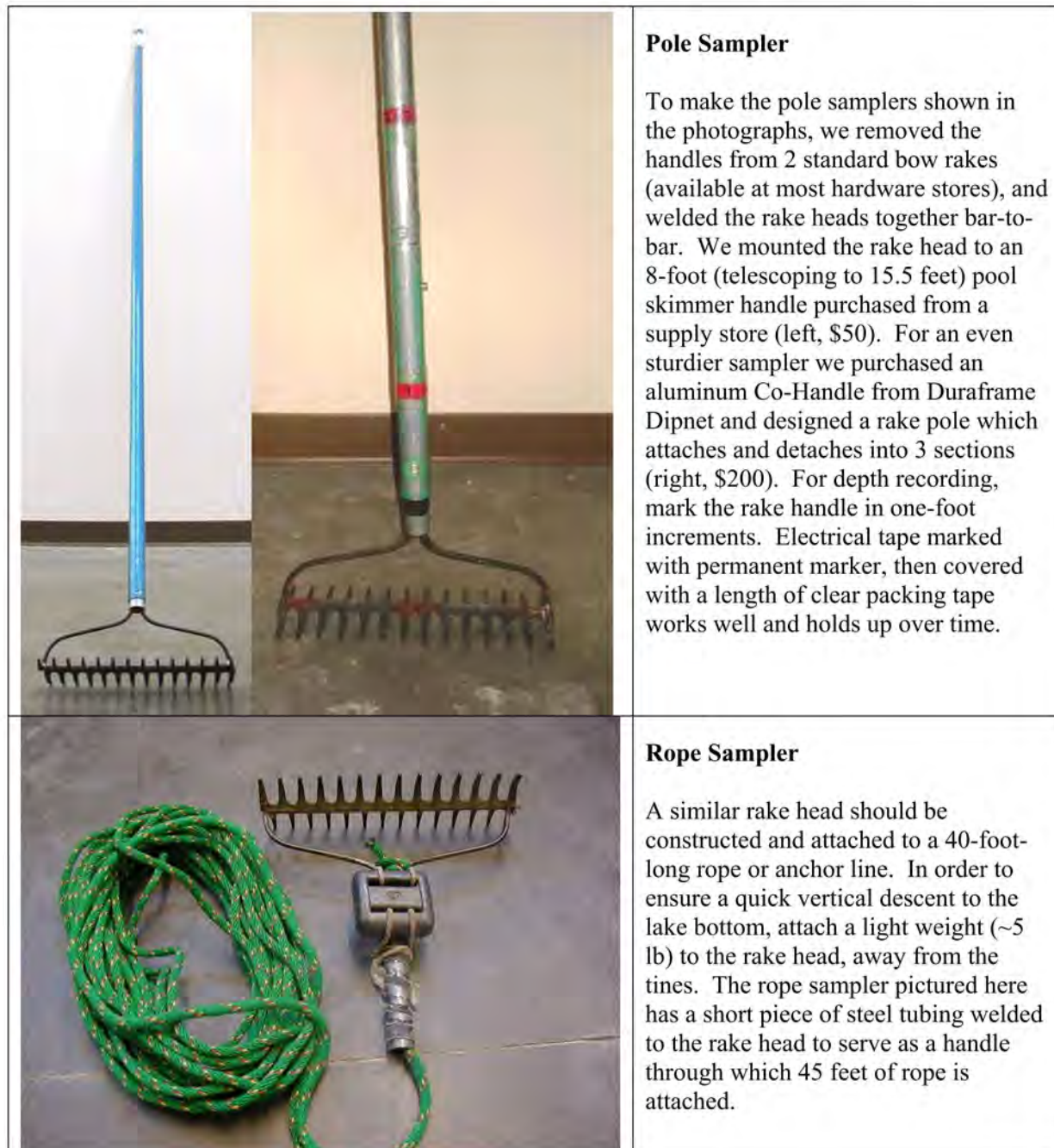
Figure 2: Examples of sampling rakes used during surveys.
